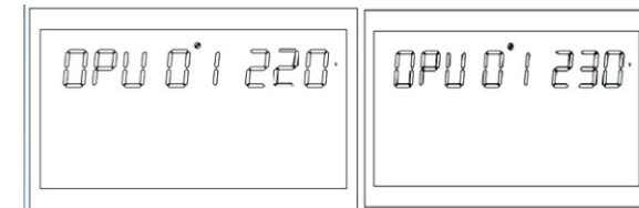
Figure 1-18 Output Voltage Setting
